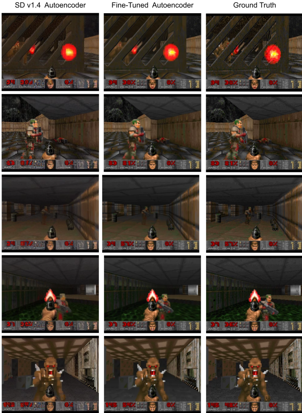
Figure 12: A comparison of generations with the standard latent decoder from Stable Diffusion v1.4 (Left), our fine-tuned decoder (Middle), and ground truth (Right). Artifacts in the frozen decoder are noticeable (e.g. in the numbers in the bottom HUD).
